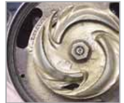
Competitor Impeller is effectively worn out.
