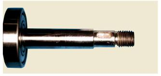
A seawater-resistant special cast iron impeller was mounted on 403 stainless steel shaft. (The shaft was protected against corrosion.)
