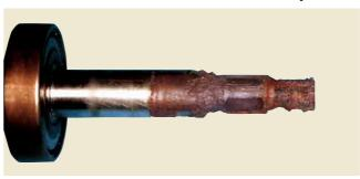
A cast 304 stainless steel impeller was mounted on 403 stainless steel shaft. (The shaft was heavily corroded.)
