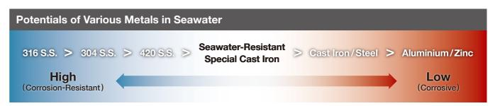
The amount of corrosive wear in the special cast iron impeller is approx. one tenth of that of conventional cast iron impeller.
